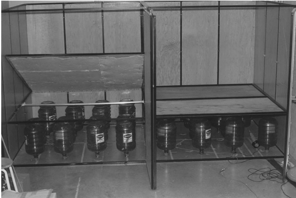
Figure 3. The fitted, 5-mFS-high, 1:8-scale model with absorbent ceiling. The front doors are open and the left roof tilted up to reveal the inside.
